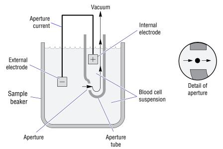
Each cell suspended in a conductive liquid (diluent) acts as an insulator. As each cell goes through the aperture, it momentarily increases the resistance of the electrical path between the submerged electrodes on either side of the aperture. This causes a measurable electronic pulse. For counting, the vacuum used to pull the diluted suspension of cells through the aperture must be at a regulated volume.
