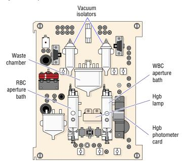
Figure 3.9 Aperture Baths and Vacuum Isolators
