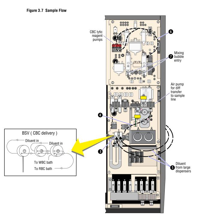
8. The BSV rotates back. The Erythrolyse II (PAK LYSE) reagent pumps send the diff lytic reagent to pick up and deliver the diff portion to the mixing chamber, rupturing red cell membranes and dissolving cell debris in the process.
